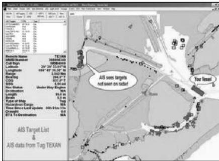
And it broadcasts plenty - directly on to your radar screen, or chart plotter or GPS screen. It will tell you, for any AIS-equipped ship within VHF-radio range, its speed and heading, which is critical in understanding if there is a threat of collision. It will also tell you when and where it will happen if both of you maintain your present course and speed (*that's when the "CPA", i.e., Closest Point of Approach, is zero...*)
