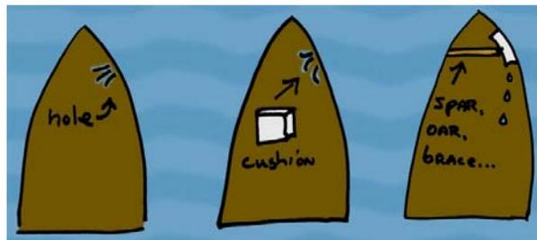
As to the other percentages and categories, roughly one in five sinkings at sea (18 percent) are due to direct leaks in the vessel itself, not caused by violent contact with the bottom or the sea itself. Areas of ingress, in order, are:
