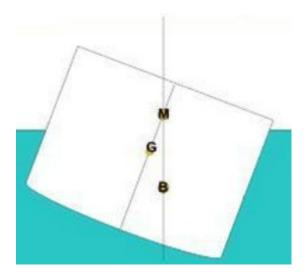
If you are starting to worry about the distance between "G" and "M", called the "Metacentric height" (or "GM" in naval architecture parlance), you're catching on quickly. The math gets pretty complicated from here, but suffice it to say that the ability of the boat to right herself (i.e, her "righting arm" or "righting moment") has a lot to do with GM. The larger the GM acting as a lever, the better.
